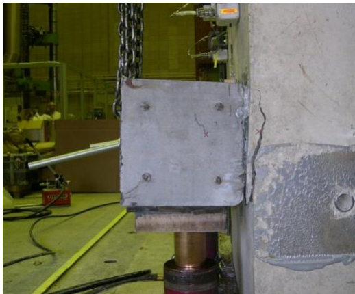
(a) Side view showing cracked abutment
