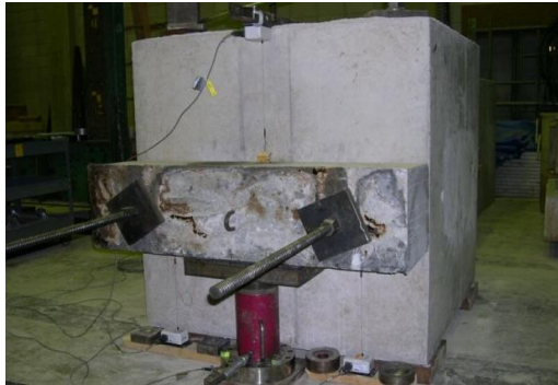
Figure 4. Assembled precast paving notch system (Phase 1).
