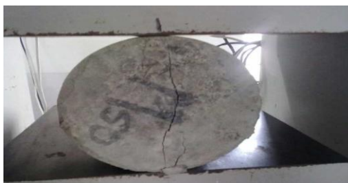
Figure. 3. Split Tensile Strength Test in Progress
