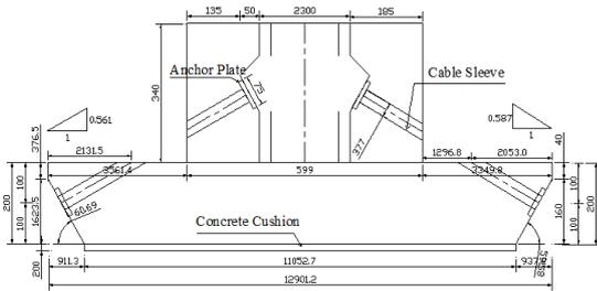
Figure 2. Details of the test model (mm)
