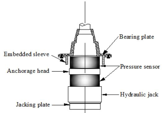
Figure 5. The installation diagram of test for anchorage head friction loss
