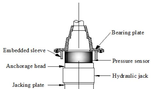
Figure 6. The installation diagram of test for anchorage head friction loss
