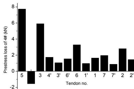
Figure 7. Loss of tendon no.4# due to concrete elastic shortening
