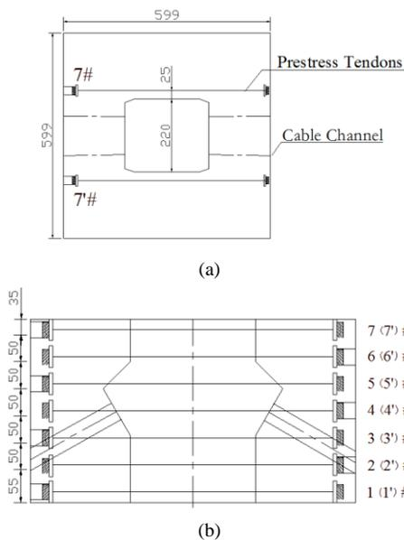
Figure 3. The layout of prestress tendons (cm): (a) plan view (b) side view
