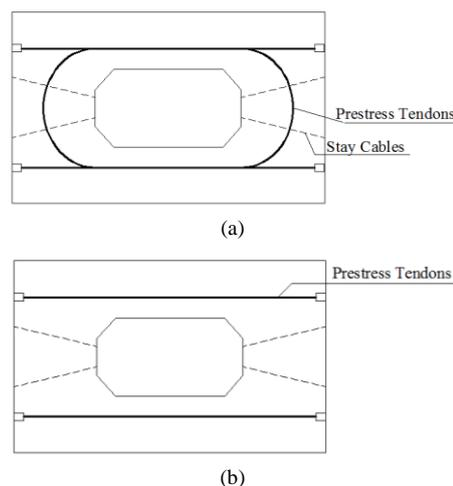
Figure 1. The way of prestress tendons layout:(a) U tendons; (b) one-way tendons
