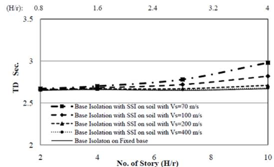
Figure 6. Damped period of isolation system considering SSI effects (Fixed base  $T_d=2.5$ s)
