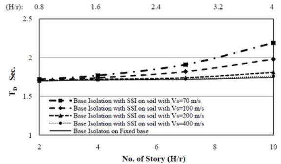
Figure 5. Damped period of isolation system considering SSI effects (Fixed base  $T_d=1.6$ s)
