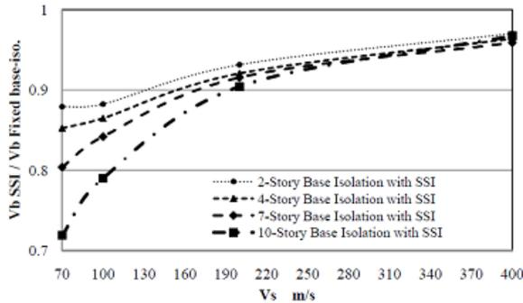
Figure 7. Ratio of base shear considering SSI effects to base shear without considering SSI effects (Fixed base  $T_d=1.6s$ )
