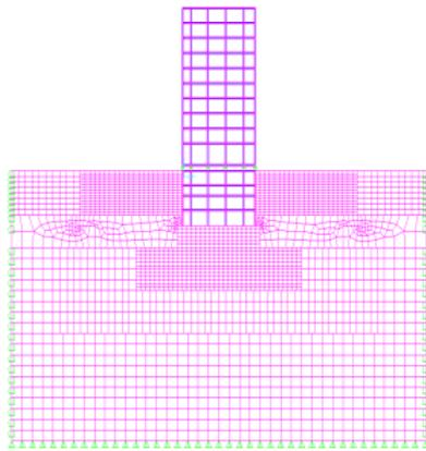
Figure 2. Finite element model of soil-structure Interaction for 2D view of building frame
