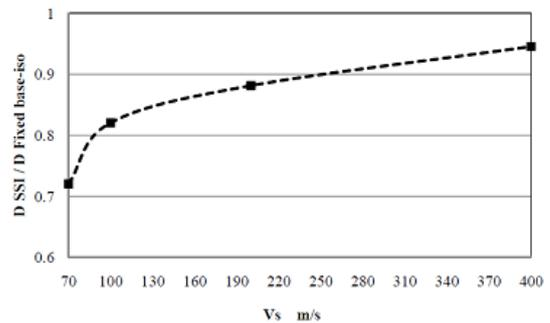
Figure 9. Ratio of total displacement considering SSI effects to total displacement without considering SSI effects
