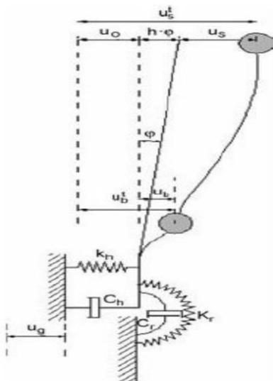
Figure 4. Analytical model of soil-structure interaction
