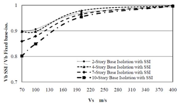
Figure 8. Ratio of base shear considering SSI effects to base shear without considering SSI effects (Fixed base  $T_d=2.5s$ )
