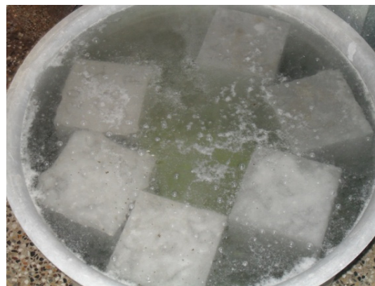
Figure 1b: Accelerated Curing (Boiling Water Curing) BWC
