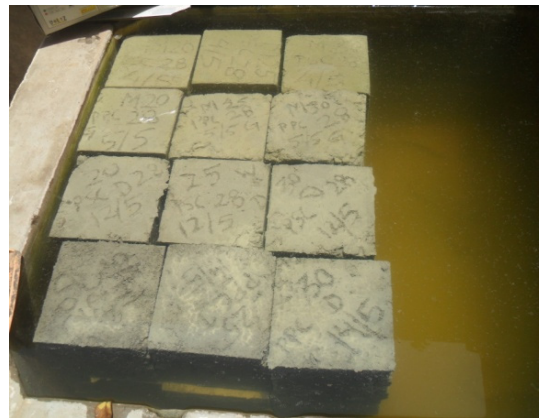
Figure 1b: Accelerated Curing (Boiling Water Curing) BWC
