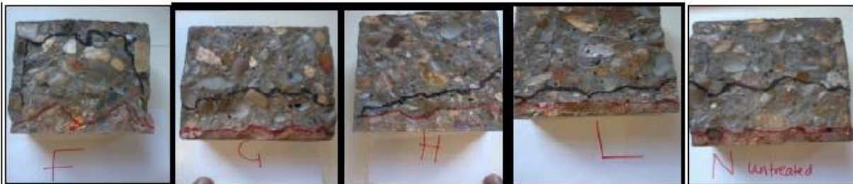
Figure 17: Dye Depth for all surface Treated Concrete Cube in Products F,G,H, L and N Respectively
