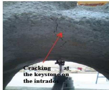
This method of reinforcement yielded the best results. Figure 34 compares all methods of reinforcement studied. The tensile strength gain was approximately 1583% that of the unlined vault, 803% that of the lined vault, 140% that of the lined vault reinforced by carbon-fibre fabric and 90% that of the lined vault reinforced by carbon-fibre strips (Figure 35).
