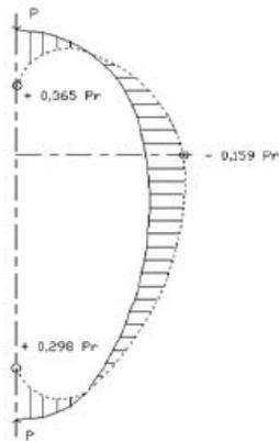
distribution of moments along the contour of an ovate structure. The maximum moment occurs at the keystone of the vault. Vertical loading denotes the vertical pressure of soils, as well as pressures due to dynamic loads such as rolling loads, permanent roads and surface construction sites. The most common failure mechanisms associated with vertical loading include a sagging vault and abutment divergence, as shown in Figure 7.
