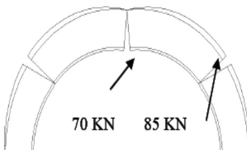
The cracks were continuous across the entire length of the vault. The vaults reinforced by strips did not undergo sagging (see Figure 23).
