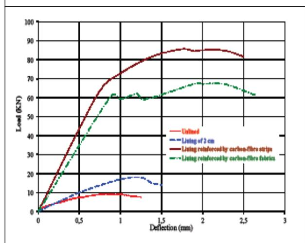
of 0.9 mm and subsequently a plastic plateau corresponding to a load of 64 kN until a deflection of 1.5 mm. Next, the load increased slightly until 67.76 kN, which was the point of vault failure. In the course of the trial, the carbon-fibre fabric became unglued at 63 kN on the intrados at the keystone. At the plateau, additional ungluing subsequently occurred at various spots on the intrados (see Figure 26). The stress was transmitted to the carbon-fibre
