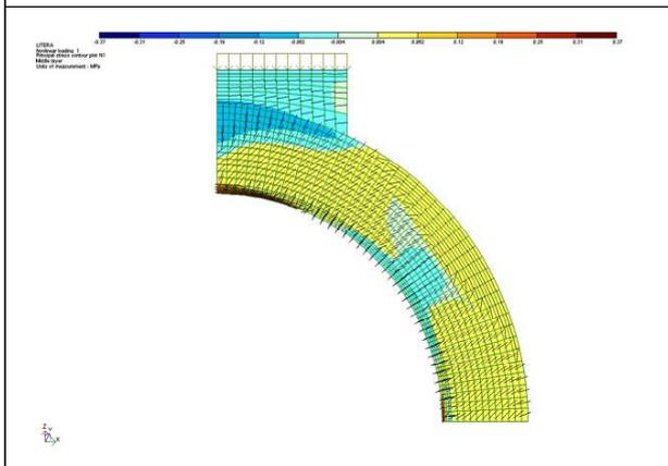
The results thus obtained show a correlation between the numerical calculations and theory. Moreover, the stresses and the displacements correspond to those of an ovoid. Tests (Kesteloot, 2005) will be conducted on vaults instead of ovoids. The dimensions of the vault used in our Finite Element Method (FEM), will be used again for the experimental campaign, with a diameter of 1.00 m and a thickness of 0.15 m.
