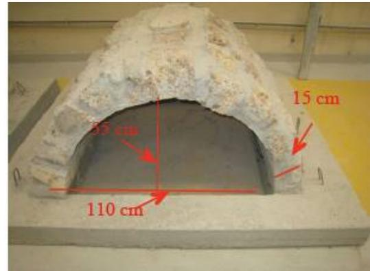
Nine vaults were constructed in accordance with the construction techniques used during the Baron Haussmann period (i.e., the mid-19th century) (Hervieu, 1897). The same mortar composition was used for all the vaults. The mechanical resistance of the mortar was monitored during vault construction. Each millstone block was unique, with different resistance and dimensions being observed.
