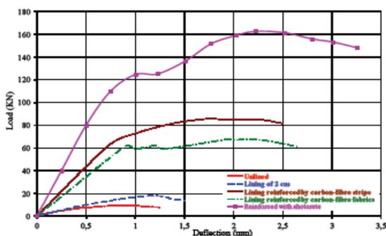
The curve shows three zones. An elastic zone is followed by a plateau up to 125 kN, which corresponds to a deflection of 1 mm. Beginning with a displacement of 1.25 mm, the behavior of the vault reinforced with shotcrete is elastic. The breaking load is 162.66 kN with a displacement of 2.25 mm. The first crack appeared at the keystone on the intrados at 110 kN (Figure 34) and continued until failure.
