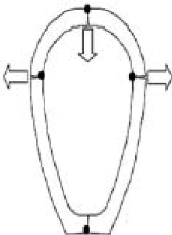
Finite element modelling was conducted by Khoufache (2008) to determine boundary conditions to ensure that the test body would be representative of an ovoid vault in real conditions. The laws of behavior which are used for masonry and coating correspond to exponential distribution (Figure 8). The loading block follows a linear elasticity model. The characteristics of the materials are given in detail in Table 1, according to the results which were obtained from tests on a building site.
