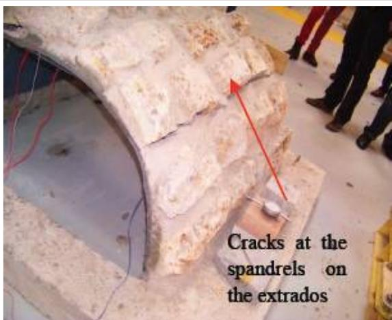
**Figure 28: Collapse of a Vault Reinforced by Carbon-fibre Fabric**
