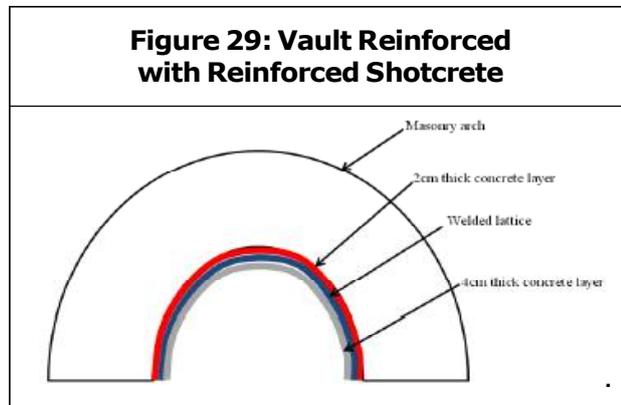
**Figure 29: Vault Reinforced with Reinforced Shotcrete**
