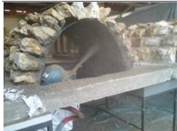
**Figure 31: Coring of the 6 x 12 cm<sup>2</sup> Samples**
