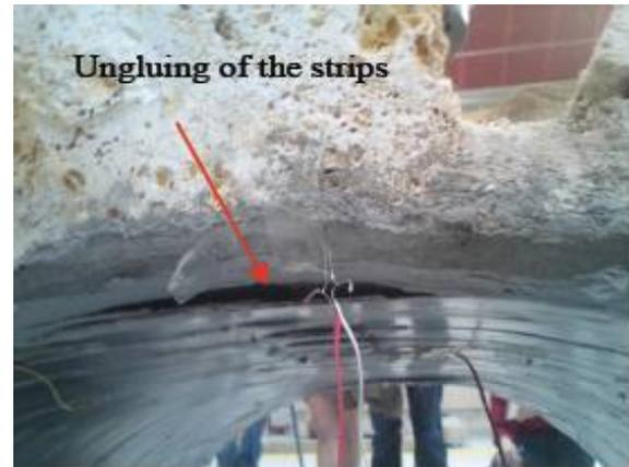
appeared both in the mortar joints at the level of the spandrels on the extrados and in the middle of the abutments on the extrados (Figures 20-22). After the breaking load of 85.85 kN, the load diminishes rapidly as the strips at the keystone on the intrados became unglued (Figure 21). The tensile strength gain is about 788% that of the unlined vault and approximately 377% that of the lined vault. The vault behavior exhibited an elastic zone followed by fragile failure.
