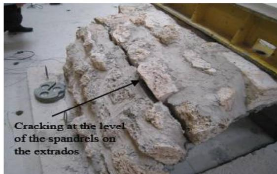
The two lined vaults exhibited the same failure mechanism.
