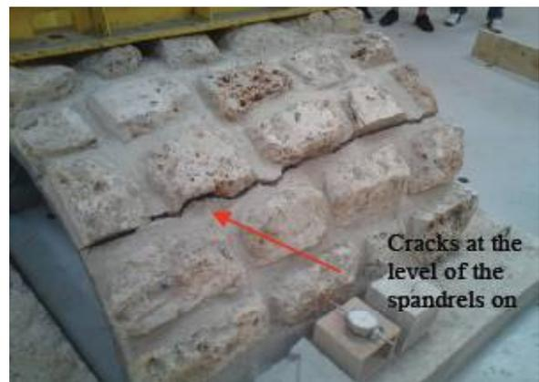
**Figure 20: Mode of Failure for the Lined Vault Reinforced With Carbon Strips**
