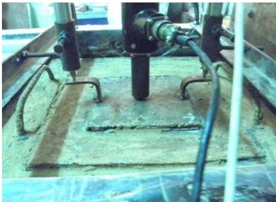
Figure 1: The Loading Frame with LVDT in Laboratory
