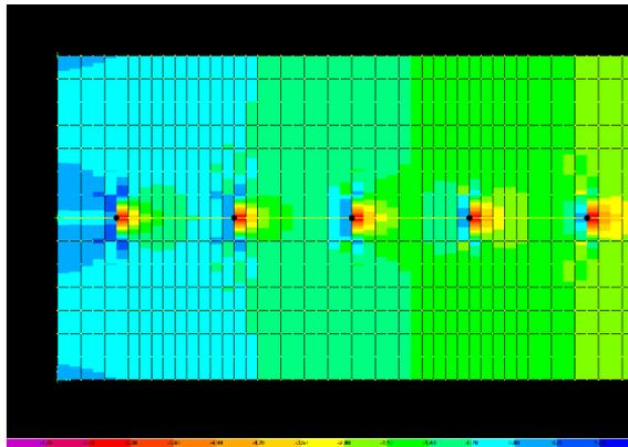
**Figure 9: Force Distributions across Concrete Slab at Four Selected Stud Locations**
