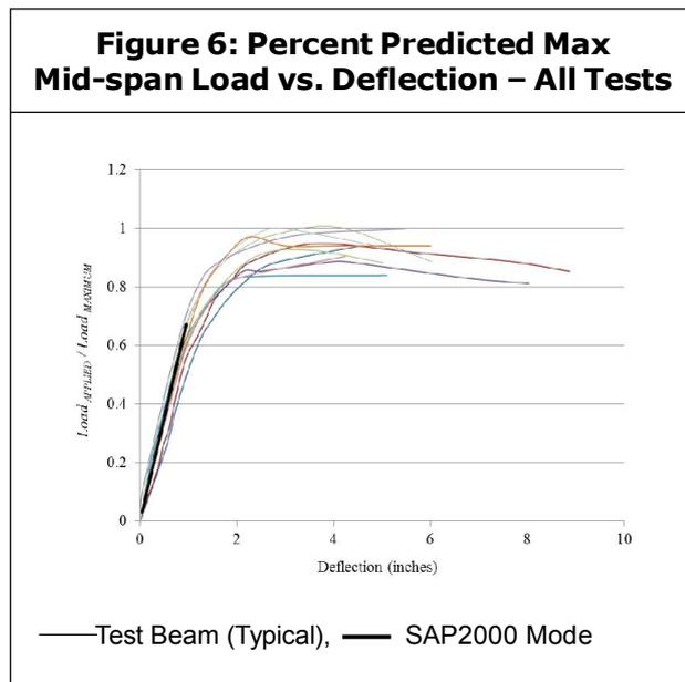
fiber must be calculated. The analytically predicted elastic limit occurs at a concentrated load equal to 21.3 kips with  $f'_c = 4,000$  psi. Observation of the test data load versus displacement graphs (Figures 7a through 7j) indicates the elastic limit occurs at a mid-span load between 20 kips and 25 kips, depending on the  $f'_c$  for the ten sets of test data.
