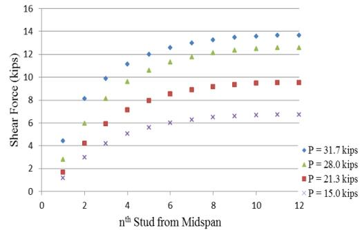
value. On this basis it can be observed that the actual maximum stud shear force may be as much as 1.25 times the predicted, uniform force. Considering the  $f'_c = 4,000$  psi case:
