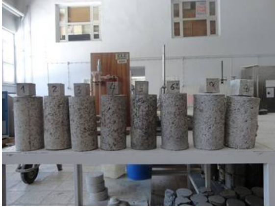
Figure 2: Volume Expansions for Geopolymer Samples Orderly (left to right 100°C-800°C)
