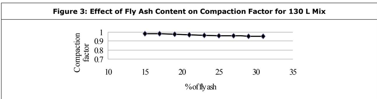
concrete is casted in to 150 X 150 X 150 mm Cubes, 150 X 300 mm Cylinders and 100 X 100 X 500 mm Prisms, to find the compressive strength, split tensile strength and flexural strength respectively. The specimens were prepared in accordance with IS-516:1959. The compaction is achieved by giving sixty manual strokes for each layer by using tamping rod and followed by compaction on vibrating table for about 30 s.
