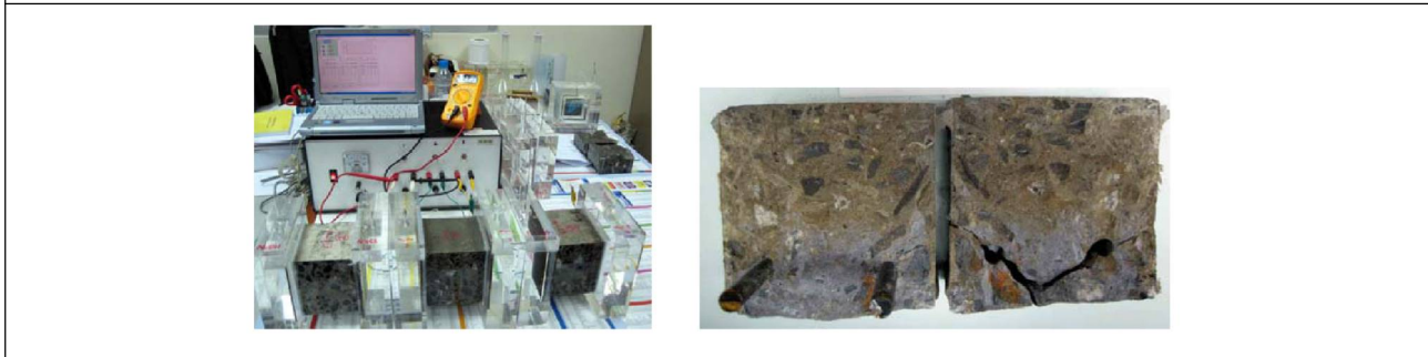
Figure 4: The Short-term Chloride Diffusion Test (A) and Chloride Penetration Depth At Cracked Concrete (B)
