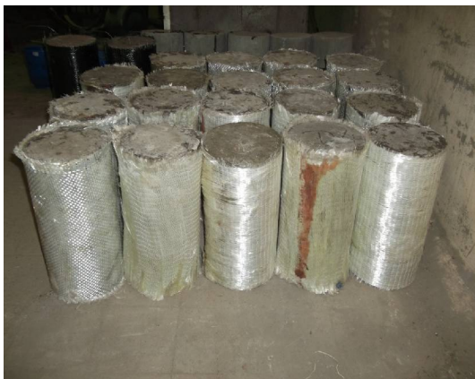
Figure 2: Failure of Unidirectional GFRP Wrapped Cylinders Along the Circumference
