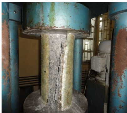
Figure 2: Failure of Unidirectional GFRP Wrapped Cylinders Along the Circumference
