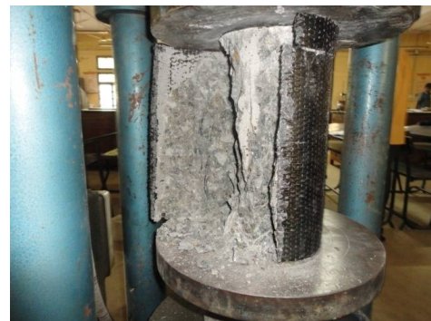
Figure 4: Failure of Unidirectional CFRP Wrapped Cylinders Along the Circumference
