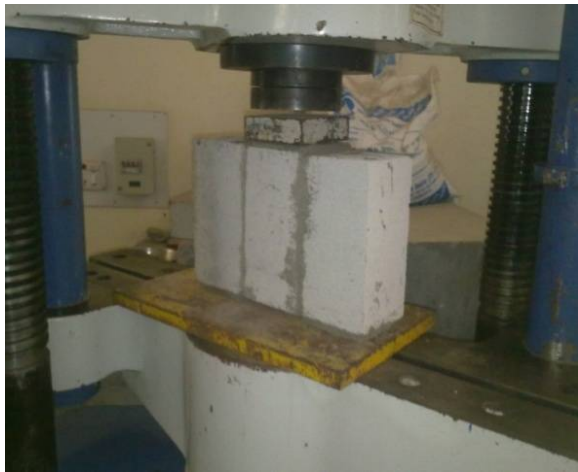
Plate 7: Triplets Shear Strength test set-up
