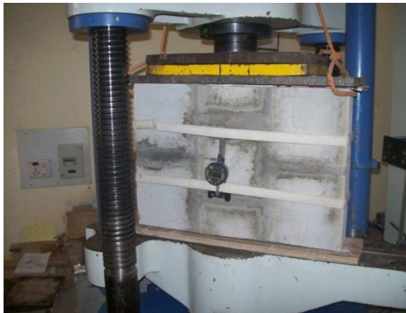
Plate 4: Set up of a typical specimen loaded parallel to bed joint
