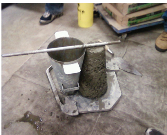
Figure 3: Slump Test on Concrete
