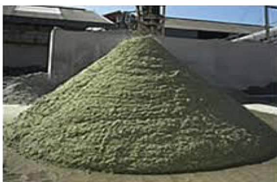
Figure 1: Waste Glass Crushed into Fine Powder
