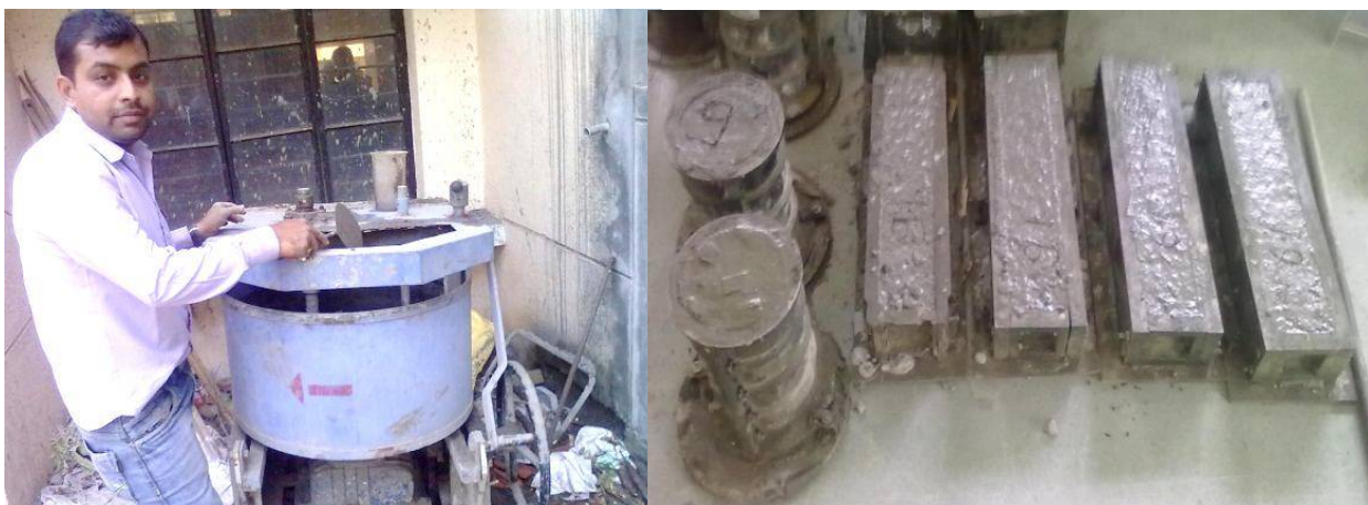
Figure 2: Rotary Drum Concrete Pan Mixer and Steel Moulds for Concrete Casting
