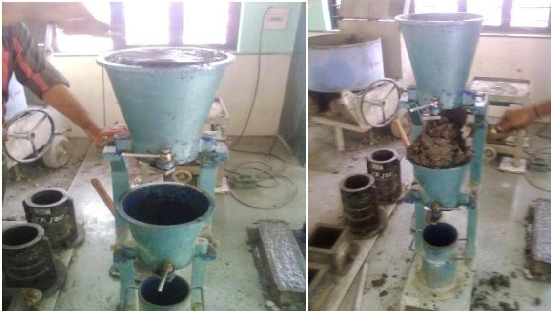
Figure 3: Compaction Factor Test for Workability of Concrete
