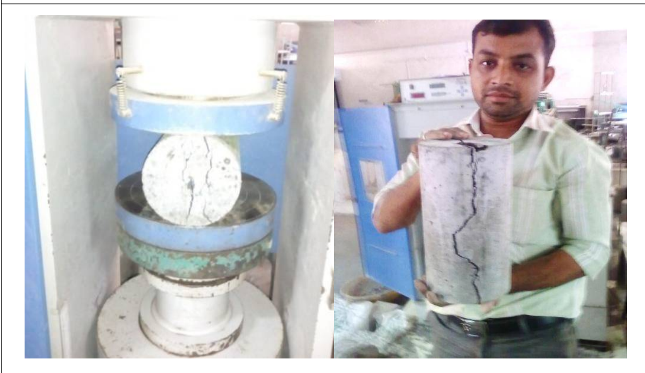
Figure 7: Testing of Cylindrical Specimen During and After Test
