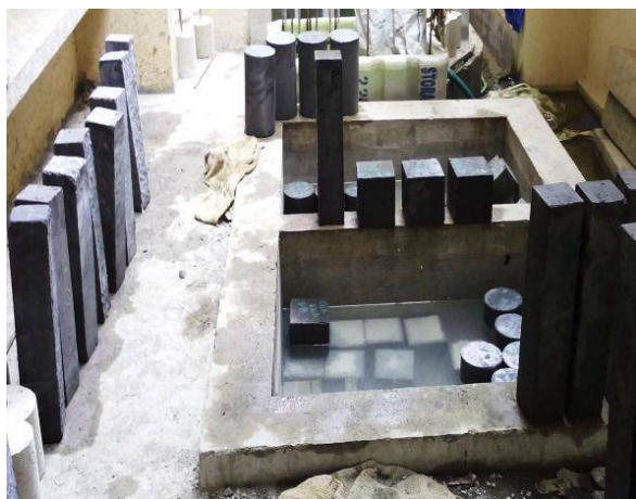
Figure 4: Curing Process of Concrete Specimens and Its Testing
