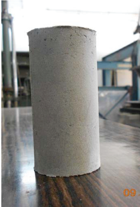
Figure 7: Triaxial Shear Test Specimen before Failure
