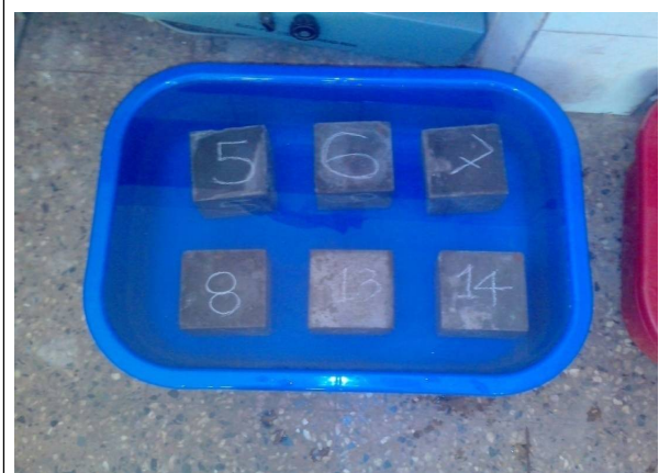
Figure 4: Specimens Immersed in H 2 SO 4 Solution
