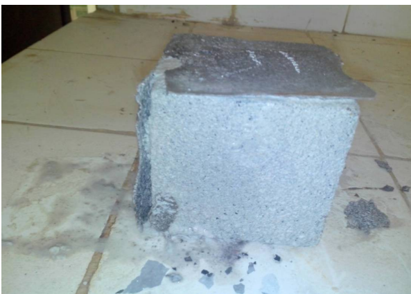
Figure 6: Surface Peels Off Due to Acid Attack
