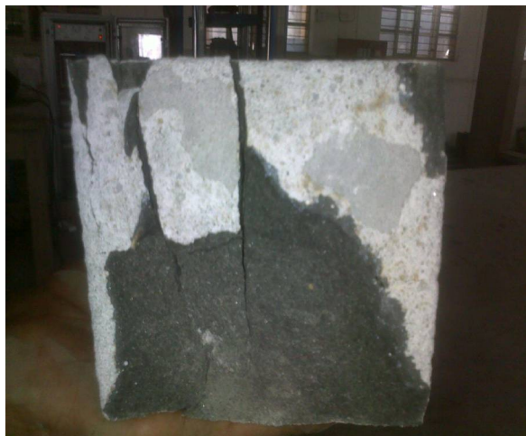
Figure 7: Fractured Surface of Specimen After Compression Test
