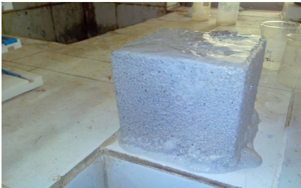
Figure 6: Surface Peels Off Due to Acid Attack
