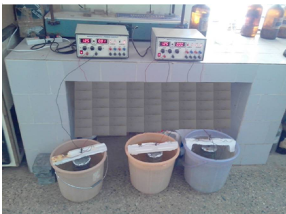
Figure 1: Accelerated Corrosion Test Setup in Laboratory
