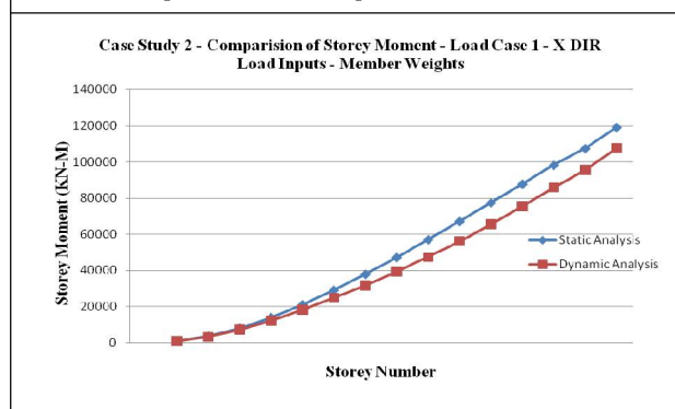
Figure 9: Comparison of Storey Moment - Static Analysis and Dynamic Analysis in X-DIR
