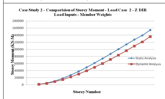
Figure 10: Comparison of Storey Moment - Static Analysis and Dynamic Analysis in Z-DIR
