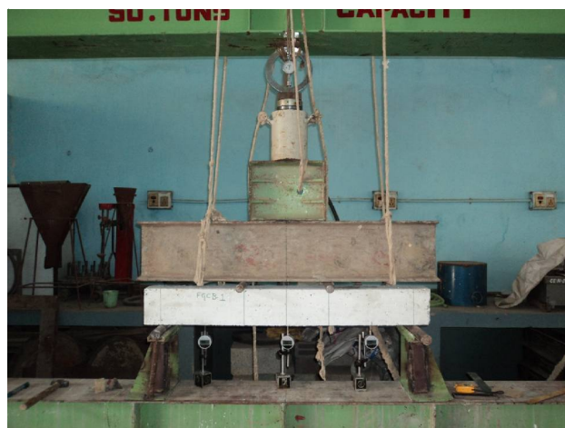
Figure 3: Arrangement Prior to Flexure Test of the Beam Specimen
