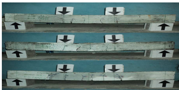
Figure 5: Crack Patterns and Failure Mode of FGC-B2 Beams
