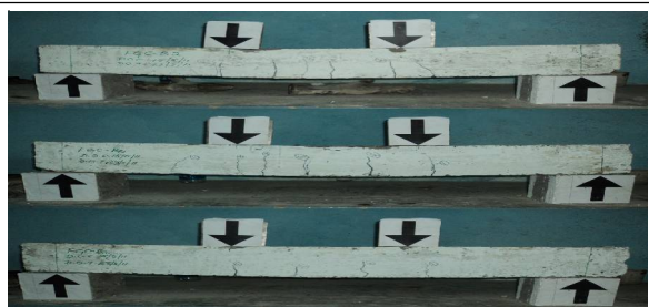
Figure 5: Crack Patterns and Failure Mode of FGC-B2 Beams
