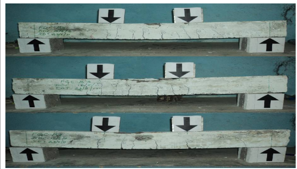
Figure 6: Crack Patterns and Failure Mode of FGC-B3 Beams
