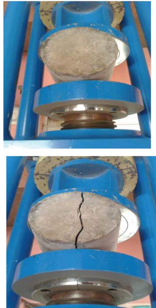
Figure 4: Split Tensile Strength Test for Cylinders
