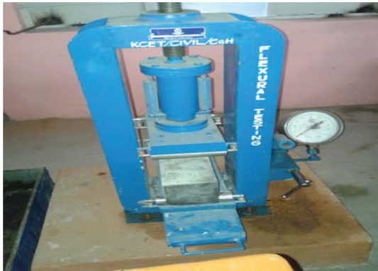
Figure 5: Flexural Strength Test for Beams
