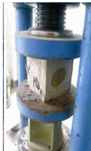
Figure 3: Compressive Strength Test for Cubes
