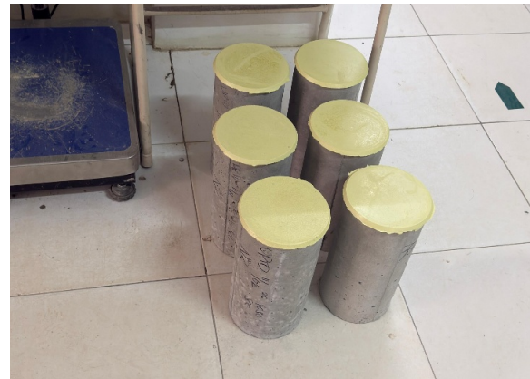
Fig. 1. Cylindrical test specimens made of Self-Compacting Concrete (SCC).
