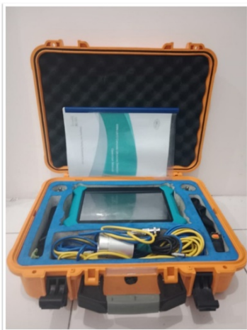
Fig. 1. Concrete Ultrasonic Pulse Velocity (UPV)-Non-Destructive Testing.
