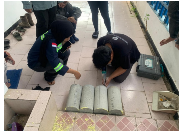
Fig. 7. Dataset for rebound testing of Self-Compacting Concrete (SCC) specimens.
