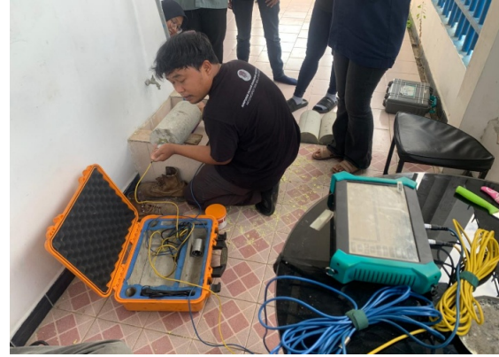
Fig. 6. Dataset for testing the ultrasonic pulse velocity of self-compacting concrete (SCC) specimens.
