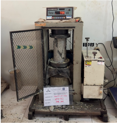
Fig. 2. Concrete compressive strength testing equipment—destructive test.
