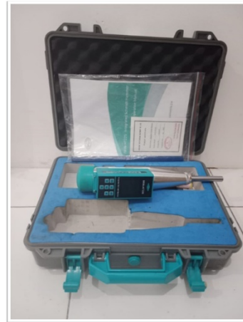
Fig. 2. IWIN-MHT225 Concrete Rebound Hammer- Non-Destructive Testing.
