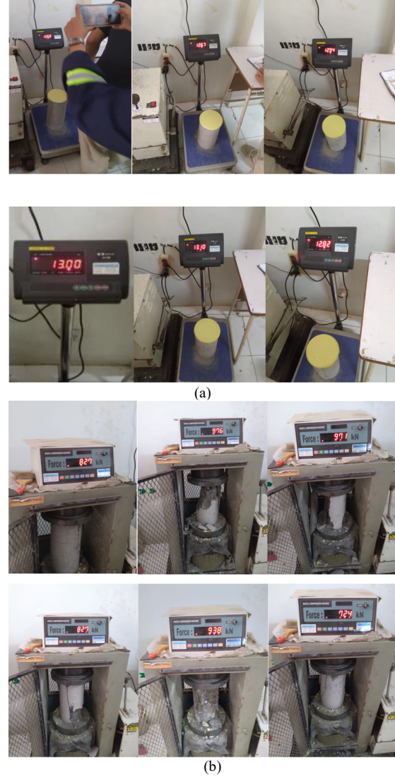
Fig. 5. (a) measurement of the weight of the test specimen (b) results of the compression test on Self-Compacting Concrete (SCC).
