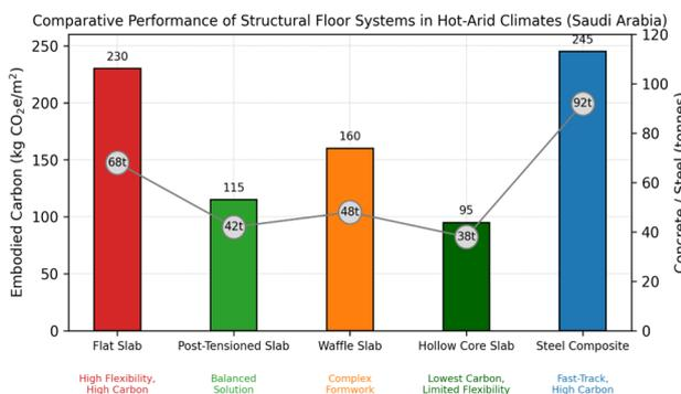
Fig. 2. Normalized embodied carbon intensity of structural floor systems expressed in kg CO<sub>2</sub>e/m<sup>2</sup>.
