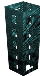
Fig. 2. FE model built-up battened column.
