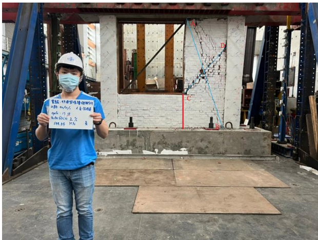
(e) Inter-story drift ratio of 2.50%
