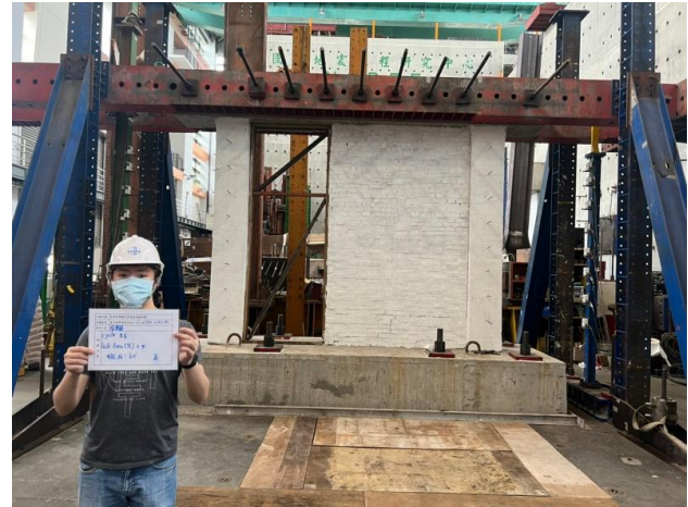
(a) Inter-story drift ratio of 0.50%
