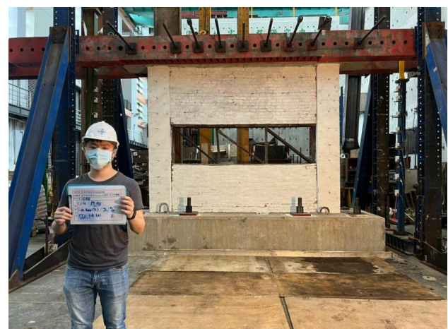
(c) Inter-story drift ratio of 2.00%
