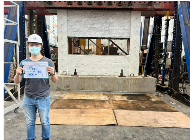
(a) Inter-story drift ratio of 0.50%
