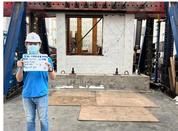
(b) Inter-story drift ratio of 1.00%
