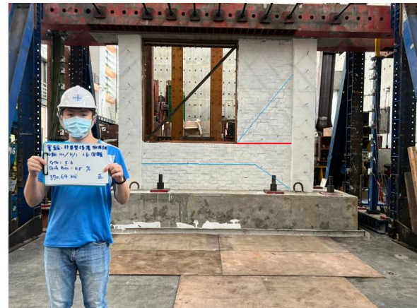
(a) Inter-story drift ratio of 0.50%
