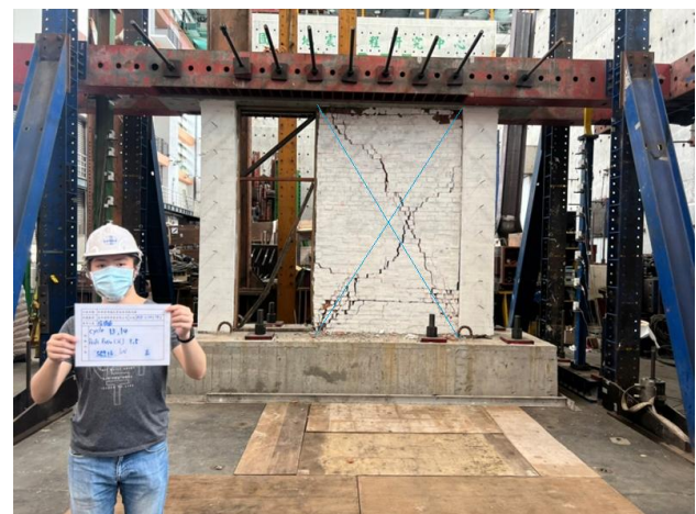
(c) Inter-story drift ratio of 1.50%
