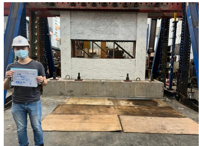
(b) Inter-story drift ratio of 1.00%
