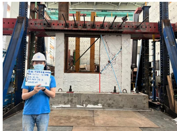
(c) Inter-story drift ratio of 1.50%
