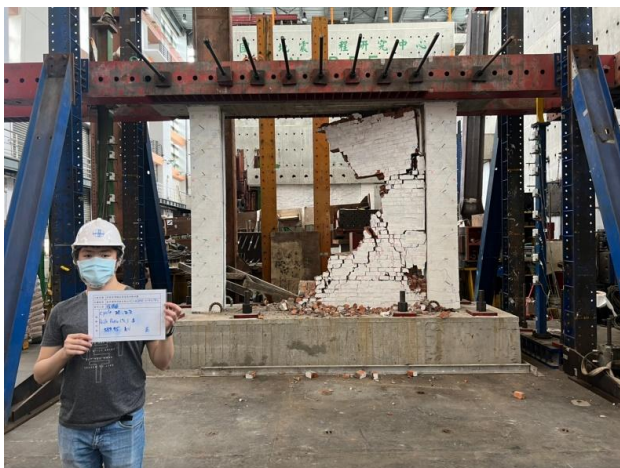
(e) Inter-story drift ratio of 3.00%
