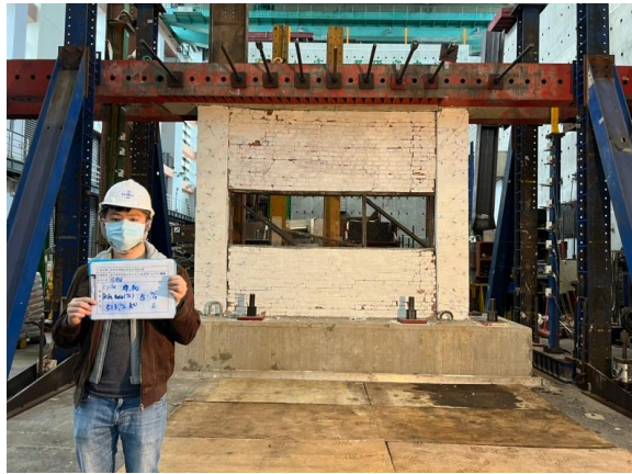
(e) Inter-story drift ratio of 5.00%
