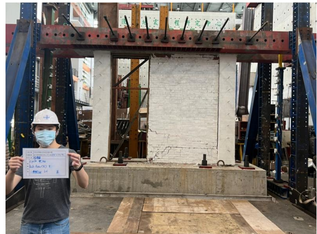
(b) Inter-story drift ratio of 1.00%
