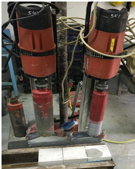
Figure 8. Absorption cores cut from cubes.
