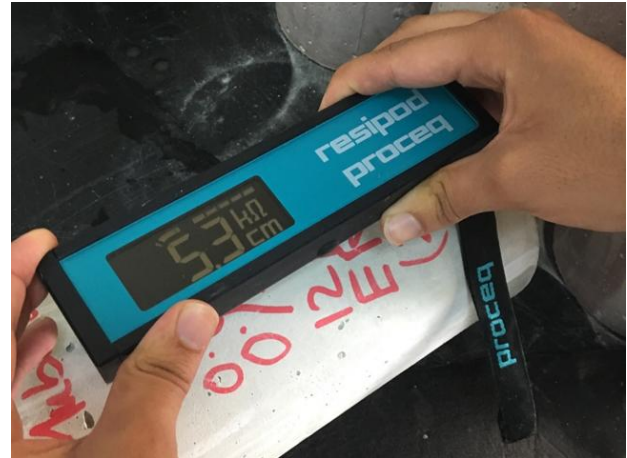
Figure 10. Electrical resistivity measurement.
